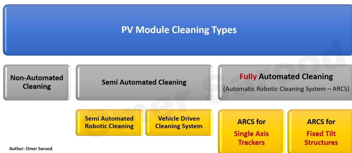
Figure 5-6: PV Modules cleaning options
